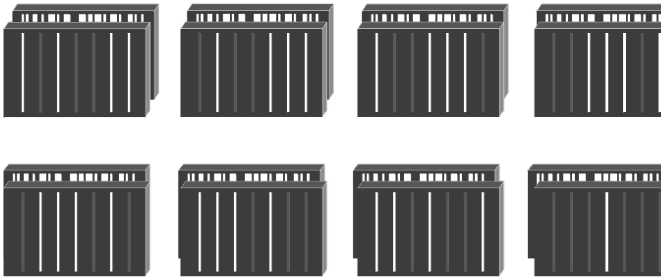
Figure 5: Switching mode of the linear slit positioning system as a spatial light modulator, two layer (two chip) architecture. The switching mode is a multiplexing mode, the HADAMARD transform mode 4 with 7 switching positions for 7 slits (switching modes are from above left to right 1010011, 0100111, 1001110, 0011101, 0111010, 1110100, 1101001, 1 is open and 0 switched off) and an additional special step for a commercial like single slit mode. The modes are generated by simple step by step shifting in the order of the slit width only.
