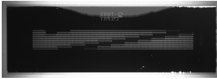
Figure 2: Two-dimensional micro-slit array (Si-chip) with 10 x 110 single slits (two-dimensional slit positioning system), top view of the 2 \mu\text{m} thick membrane (REM picture). The chip is used as an entrance slit array, illuminated is a part of 10 x 10 slits for an imaging architecture to generate 10 x 10 subpixels by a simple multiplexing mode.
